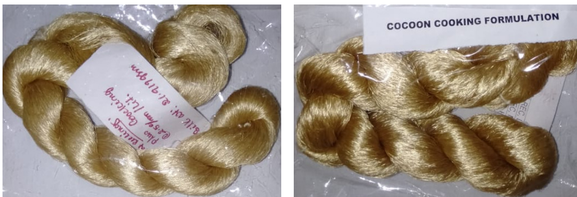
Fig. 3 : Visual comparison of silk yarn reeled using soda and new formulation respectively. The retention of natural luster in new method (right) can be clearly visualized
